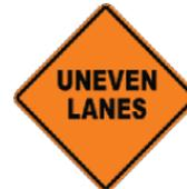
*Construction work may have caused a difference in the elevation of parallel traffic lanes.*
