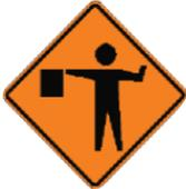
*Used at locations along a roadway where a flagger may be stationed to control traffic.*
